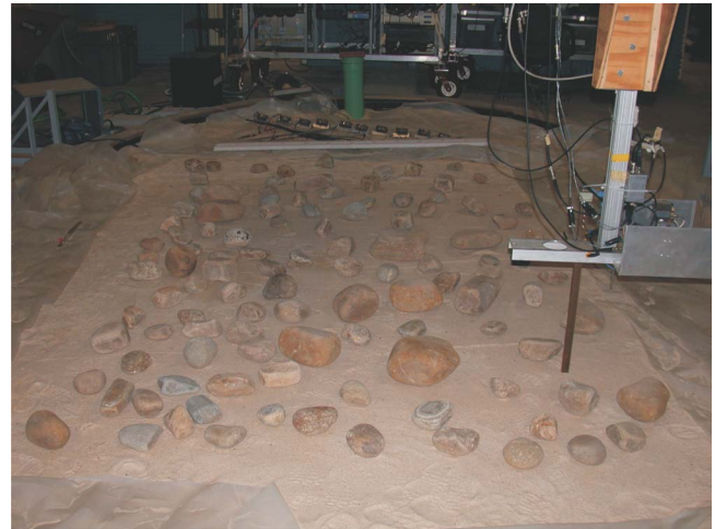
FIG. 4. (Color online) The layout of the rocks before being buried below the surface.
